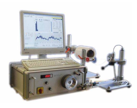
Convenient and reliable examination of the unwinding behaviour of a yarn bobbin demands for a versatile instrument, which allows for accurate recording of the whole range of forces acting on the yarn during the unwinding procedure. This allows for thorough analysis of the impact of various factors such as unwinding speed or package shape on the built up tension during unwinding.
