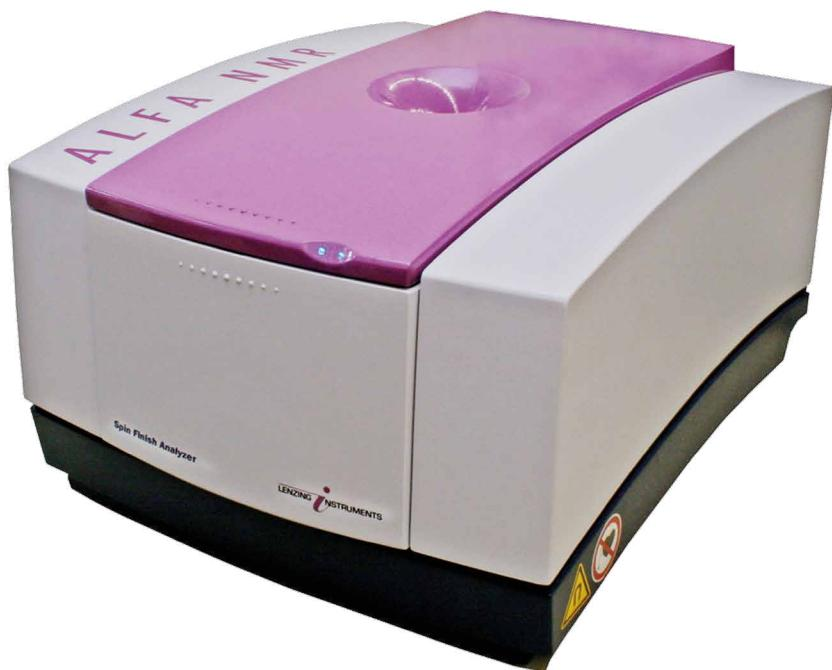
As an alternative to the spin finish analyzer ALFA 500, Lenzing Instruments offers also the **ALFA NMR**, which is based on the technique of Time Domain NMR (Nuclear Magnetic Resonance)
