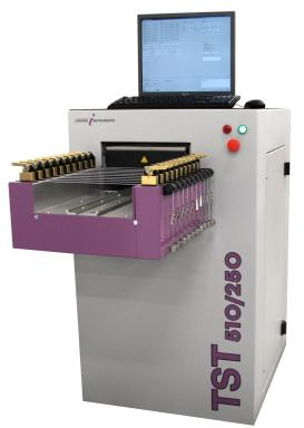
Percent shrinkage and shrinkage force at specified temperatures are two dominant quality parameters of technical and industrial yarns such as tire cord, of filament and spun yarns for textile applications as well as of plastic tapes.
