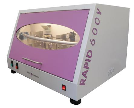
The quality of interlaced (entangled) yarns is determined by the number of nodes over a certain length, by their regularity and their tenacity, which is an essential criterion for the behaviour of the filament during downstream process steps such as weaving and knitting.
