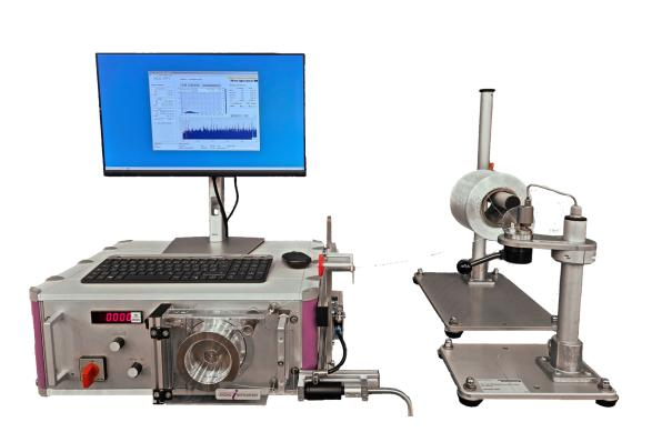
Convenient and reliable examination of the unwinding behaviour of a yarn bobbin demands for a versatile instrument, which allows for accurate recording of the whole range of forces acting on the yarn during the unwinding procedure. This allows for thorough analysis of the impact of various factors such as unwinding speed or package shape on the built up tension during unwinding.
