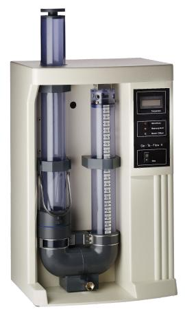
The **GE-TE-FLOW** Permeameter is a fully automatic, computer-controlled instrument for testing the water permeability of geotextiles, fleeces and related materials. In conformity with EN ISO 11058, it operates by the falling head method, measuring normal to the specimen plane and without a load applied.
