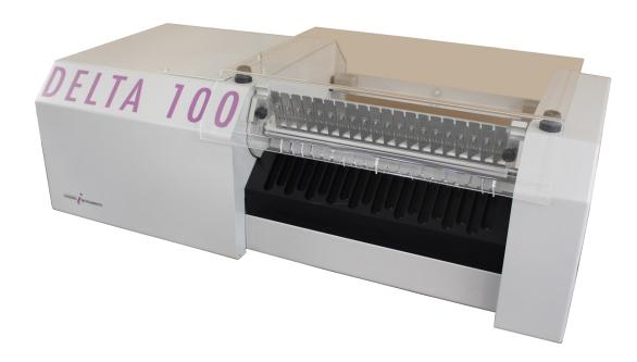
A precise characterization of the abrasion properties of single fibers in the wet state enables an estimation of their fibrillation tendency. Therewith, the strength of the fibers in further processing and the haptic properties of end products can be predicted.
