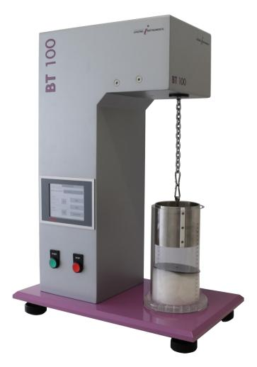
The comfort and functionality of pillows and similar end products are characterized by their firmness, capacity to retain shape and to give support. By testing filling materials like staple fibers for their compressibility, filling power and recovery properties, the requested comfort can be determined and accomplished.
