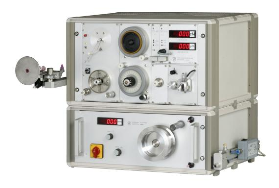
During filament yarn production, unintended abrasion due to various parameters such as yarn twist, yarn titer (dtex, den) and wax levels may cause production downtime. An exact quantification of the abrasive yarn characteristics gives information both of the unintended abrasion as well as of the positive, abrasion-reducing properties of spin finish oil.
